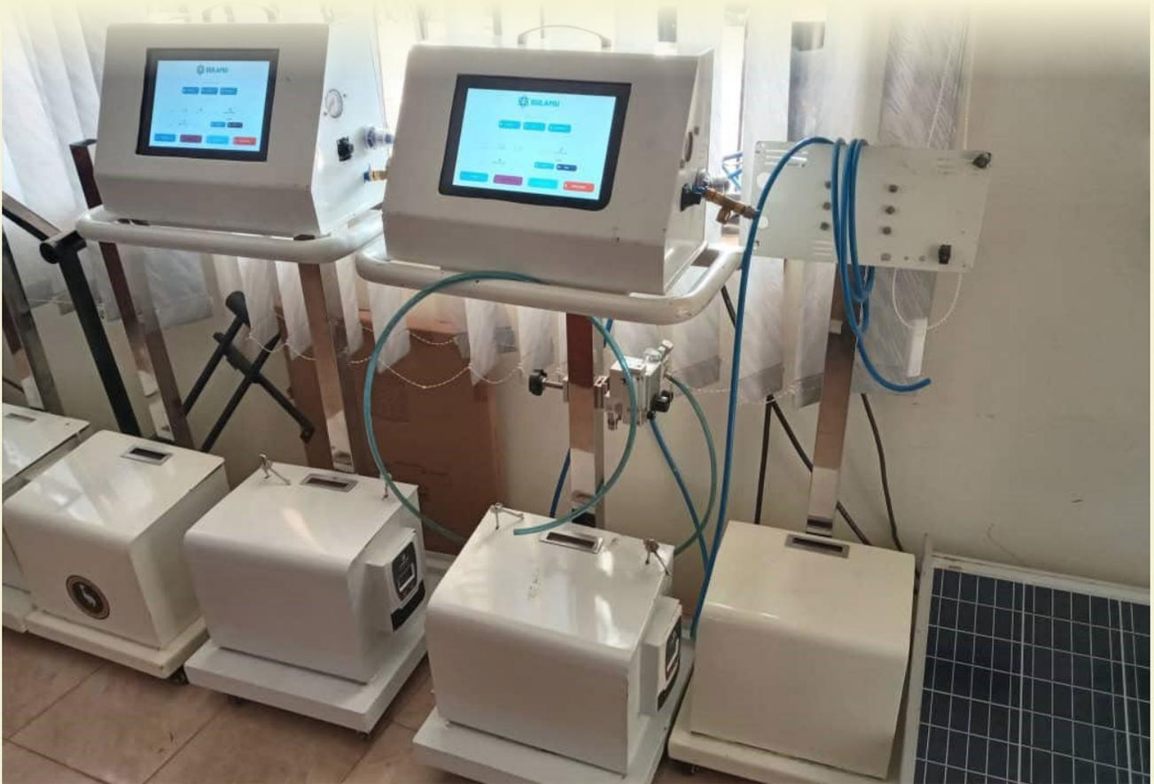
*The two Bulamu low-cost medical ventilators assembled and ready for animal tests*
